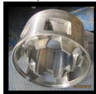
Variable Resistance Trim ( VRT ): Linear
