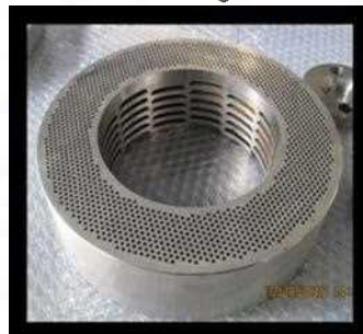
Variable Resistance Trim ( VRT ): Linear
